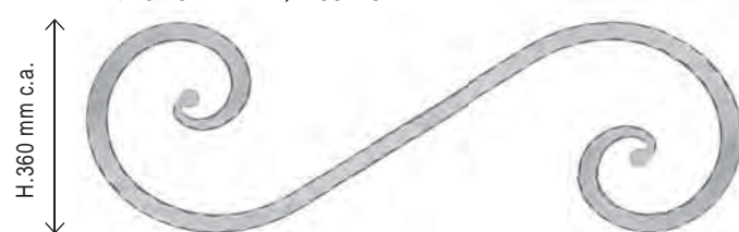
Sinistro / Left Martellato / Hammered H. 360 x L. 1500 mm. Art.15.157.224 \neq 30 x 8 mm
